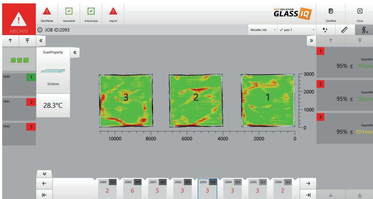
Exemplary anisotropy images of our sedak scanner with 3 glasses in one batch rated by the corresponding 95% quantile value.
