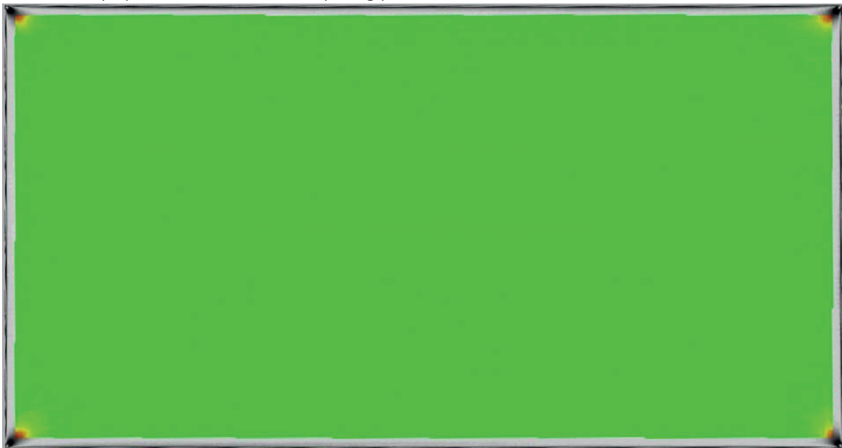
Anisotropy scan of a 6m x 3,2m 10mm sedak tempered+ with a 95% quantile value of \leq 60\text{nm} .
